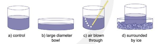
The control will show the rate of cooling due to classroom conditions, e.g. temperature. The water in b, c and d cools faster than the water in a. In b and c the water is exposed to a larger surface area of cool air (provided by air bubbles in c), and in d the water is exposed to a colder surface. Allow the children to offer explanations of their results whilst ensuring that the discussion covers the factors mentioned above.
